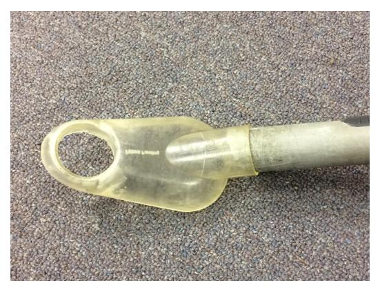
Bit Buddy Shroud attached to a HEPA vacuum
