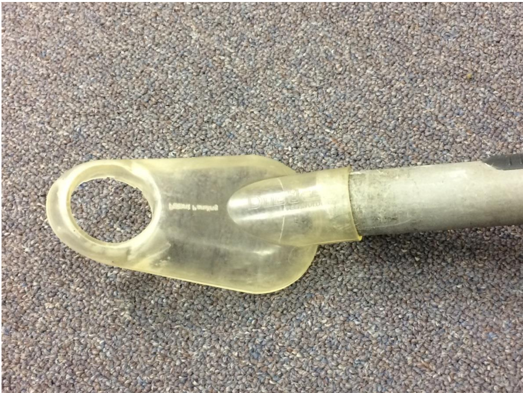
Bit Buddy Shroud attached to a HEPA vacuum
