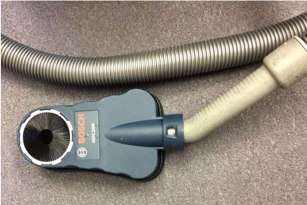
BOSCH HDC200 Shroud attached to a HEPA Vacuum
