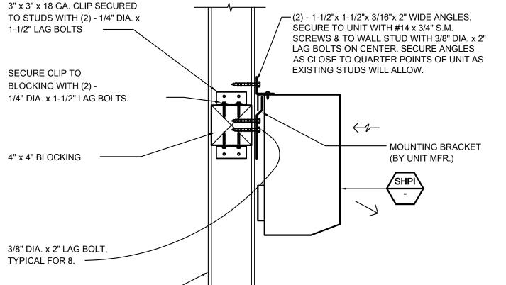
INDOOR SPLIT SHPI UNIT MOUNTING 3 **M5**. SCALE : NONE
