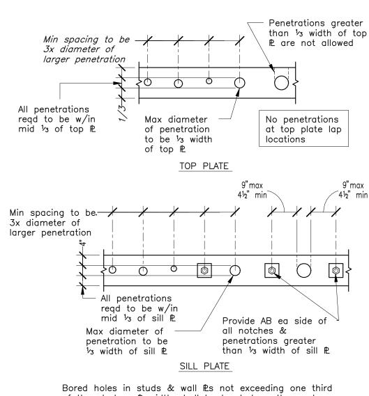
of the stud or P width shall be located on the centerline of the member being penetrated & at a minimum spacing of 12" & 12" from end of stud or wall P. Bored holes at studs to occur @ 3 max consecutive studs.
