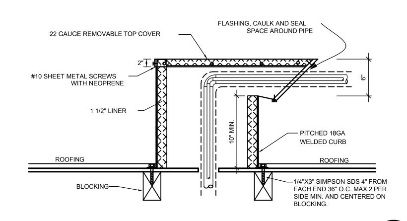
PIPE THRU ROOF SAFE DETAIL - WOOD
