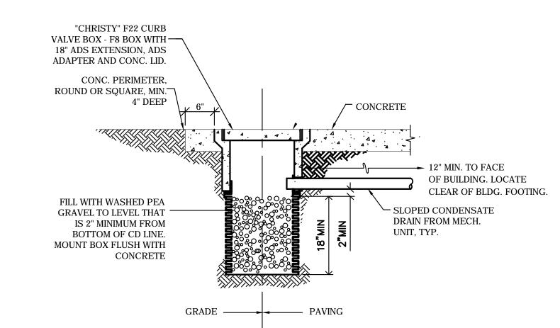
ROUTE CONDENSATE DRAIN THRU WALL AS LOW AS POSSIBLE AND DROP TO BELOW GRADE AS SOON AS POSSIBLE.
