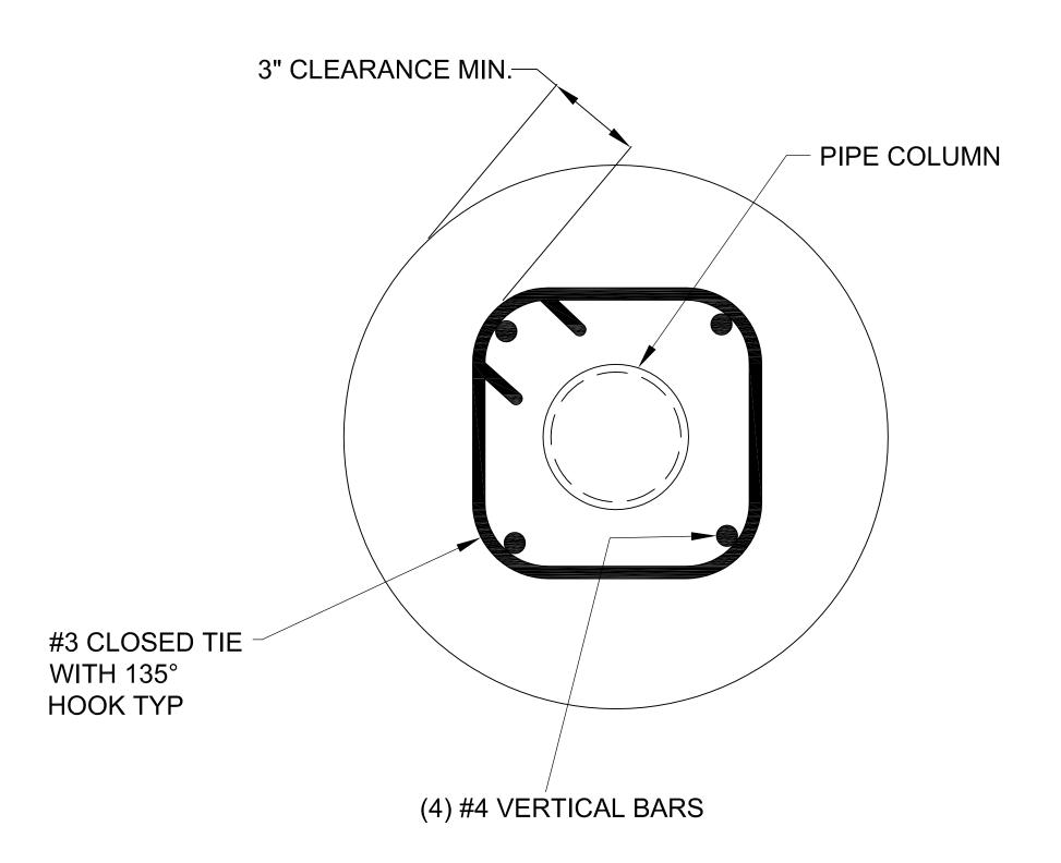
TYPICAL PLAN VIEW OF FOOTING DETAIL
