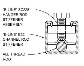
FOR 3/8" THRU 5/8" ROD (FOR 3/4" & 7/8" ROD USE SC-UB)
