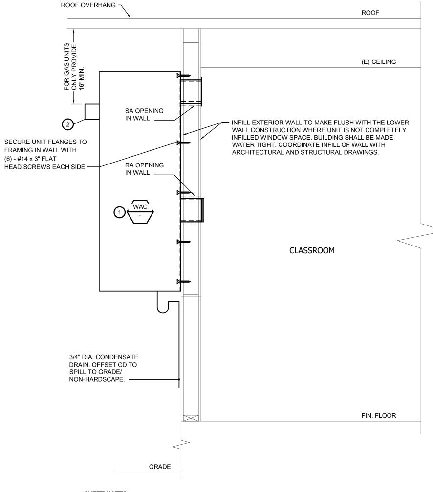
1 REMOVE (E) WALL MOUNT UNIT AND REPLACE WITH (N) WALL MOUNT UNIT BY BARD MANUFACTURER.
