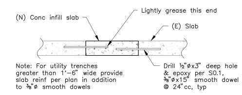
(N) Slab to (E) Slab @ Utility Trench S0.3
