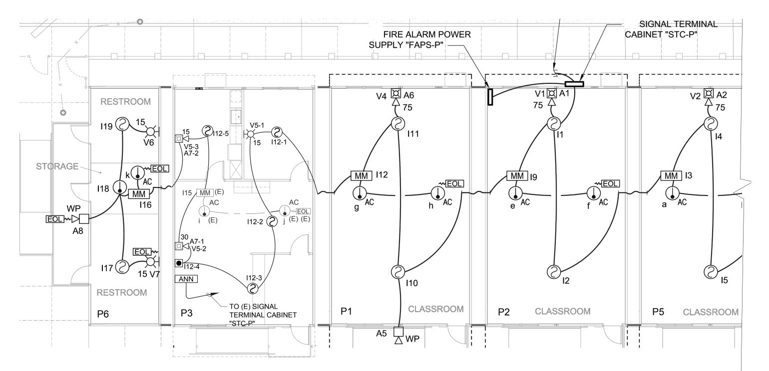
ALL DEVICES SHOWN IN BUILDINGS P6, P1, P2, P5 IS EXISTING AND IS SHOWN FOR REFERENCE. DEVICES IN BUILDING P3 IS NEW EXCEPT WHERE SHOWN.
